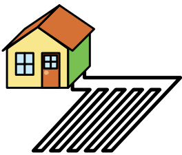
Horizontal Closed Loop: 4 ft. deep
